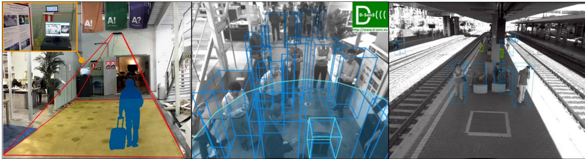
Figure 5: Left-item detection in scene based on combining depth and intensity information. Left: the demo scenario at UrbanMill used for demo session over many months. Center and right: Detected scene objects (blue – persons, green – stationary left item candidates, circle – vicinity for owner detection) in an indoor and outdoor environment.
