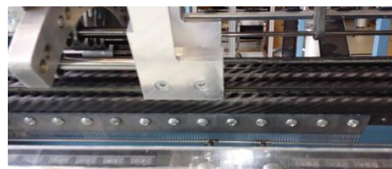
Figure 2 - Pattern bar and stem parts on Alge machine (frontal)
