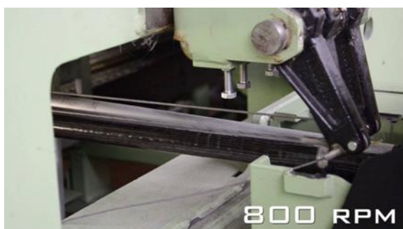
Figure 1 - Push rod on a Selcom machine (frontal)
