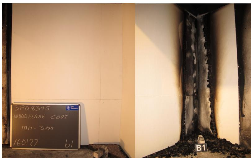
As can be seen in the table above, the coating MH-m-ox achieved 2 of 3 parameters for Class C-s1,d0 according to classification standard EN 13501-1. Only parameter THR was not fulfilled.
