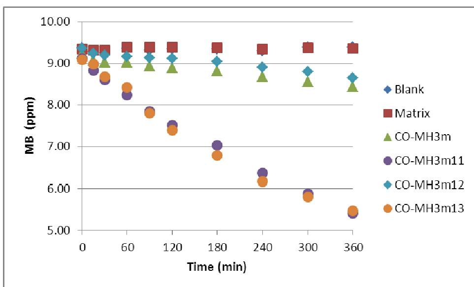
Maximum degradation rate occurred for the CO-MH3-m11 and CO-MH3-m13 coatings, due to the presence of TiO<sub>2</sub> and ZnO nanoparticles.
