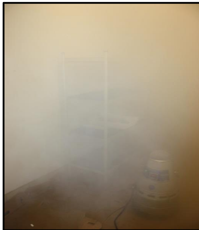
Figure 3: Fog formed into the chamber during AEROBRUMER application.
