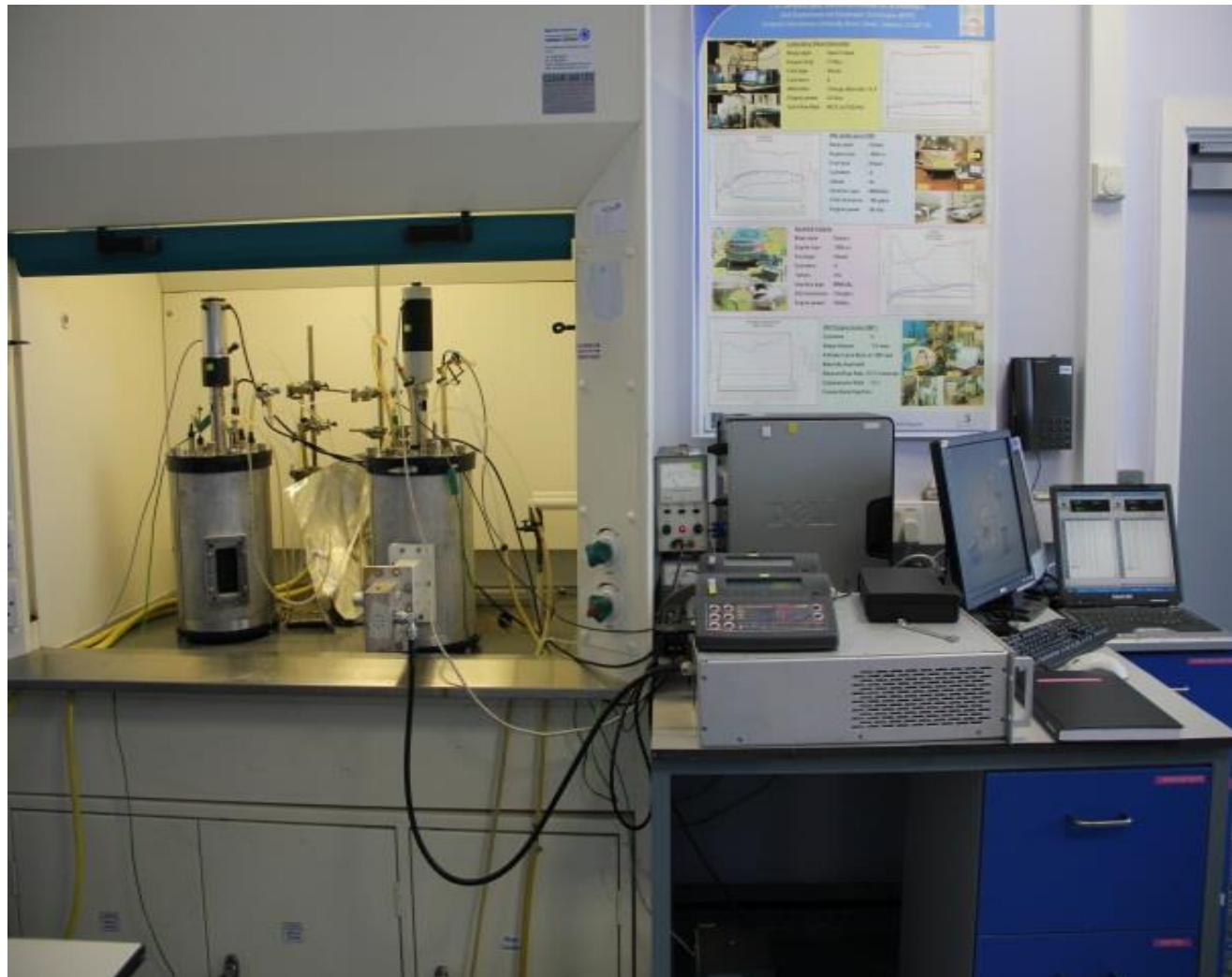
Complete system with microwave source, automation and control of parameters
