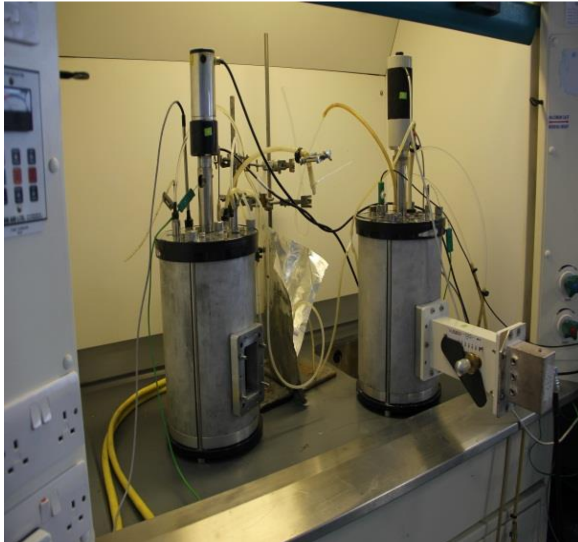
10 L Microwave plasma reactors with and without pig manure
