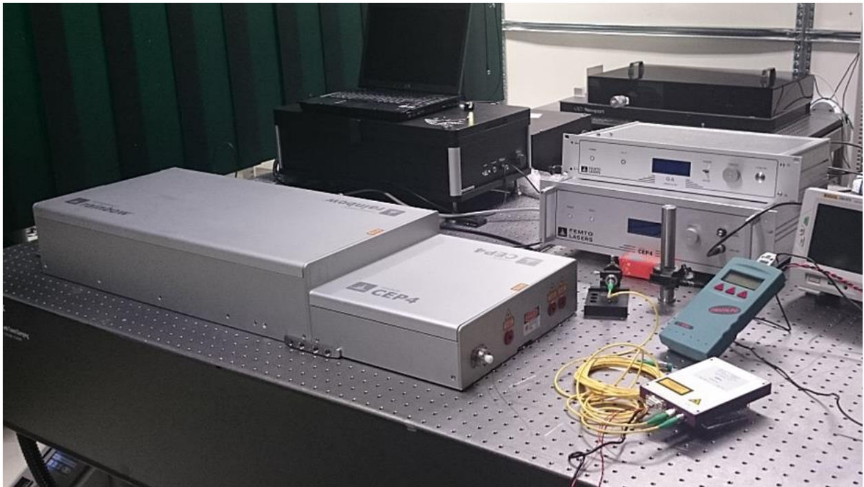
Fig. 3: The laser head contains the Ti:sapphire cavity, the pump laser, adjustable glass wedges, photo diodes and electronics. It is attached to the CEP module that provides both a free-space and a fiber coupled output.
