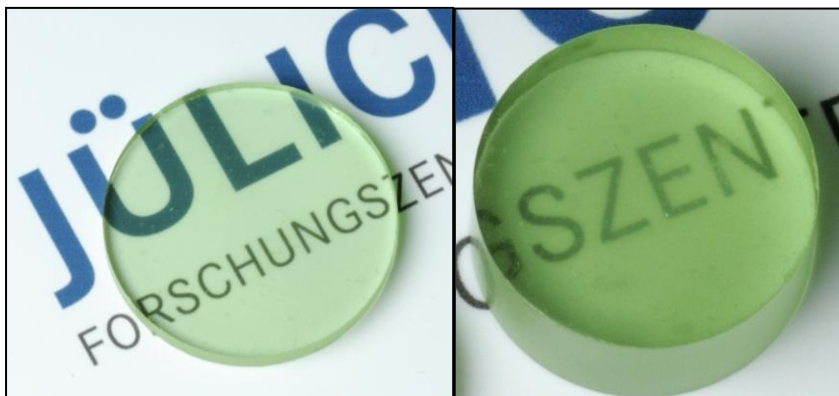
Figure 1a: Transparent ceramics of YAG:Pr with different diameter and thickness (left: \varnothing 3.2 cm, h: 2 mm; right: \varnothing 2 cm, h: 9 mm)
