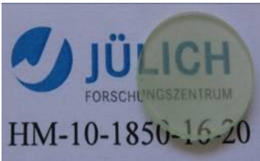
Figure 1b. Transparent LuAG:Pr as prepared in the project ( \varnothing 3.2 cm, h: 2 mm)
