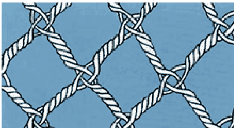
Figure 19. Twisted knotless netting diagram
