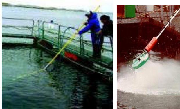
Fig. 3. Manual cleaning of cage nets using water jet device.
