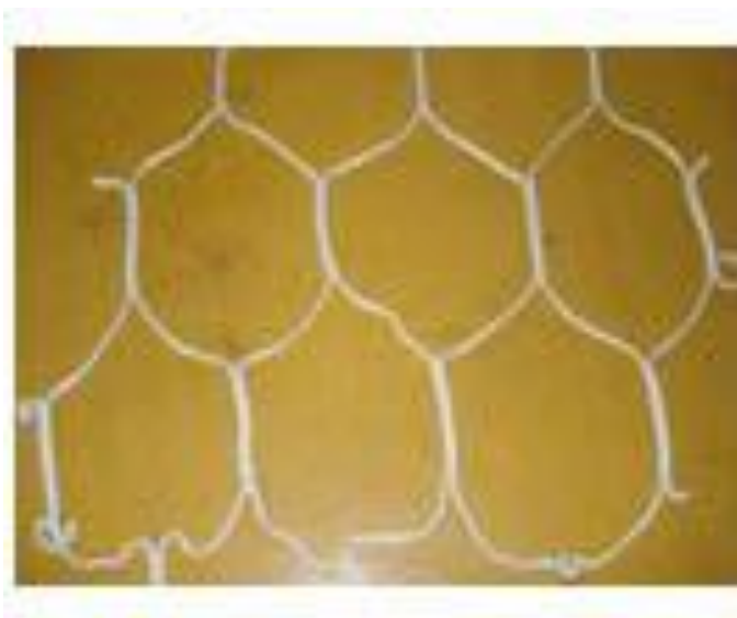
Figure 18. Hexagonal Raschel knitted mesh.
