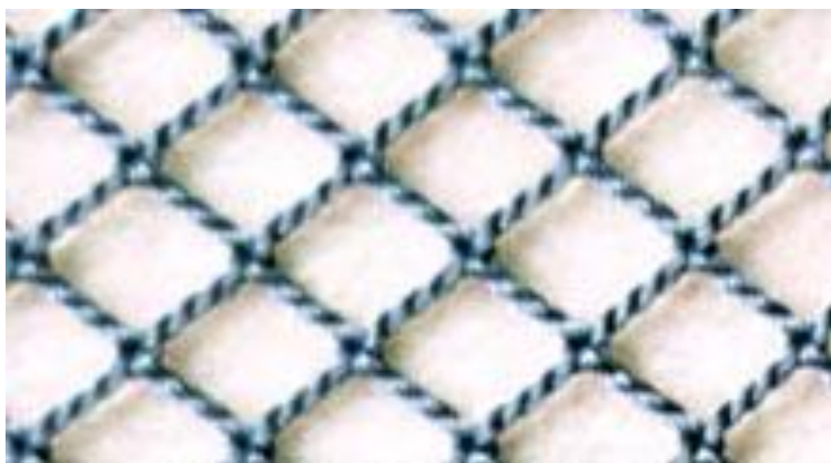
Figure 20. Twisted knotless netting from yarn
