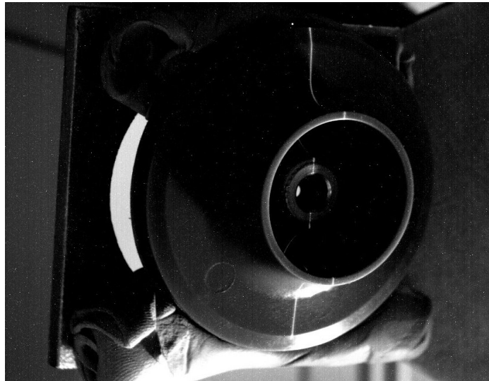
Line of COS 405 nm laser on Askoll plastic wheel (room lights on)
