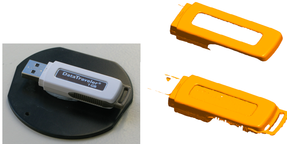
Scanning of object with non-homogeneous reflectivity (left). Top right: traditional scanner; bottom right: With OP3MET line generator.
