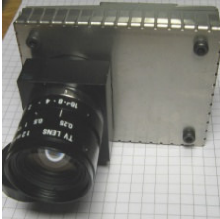
The boxed camera from front with lens mount and lens. The box shields electromagnetic emission.
