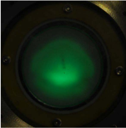
Figure 32 Transmitted beam imaged on the fluorescent screen (Salford UHV tests).
