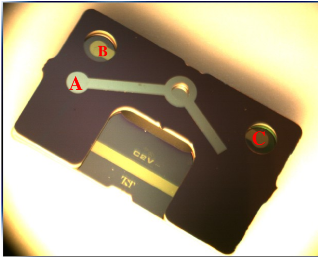
Figure 20 Photo showing the detector-facing side of the chips with contact points A, B & C
