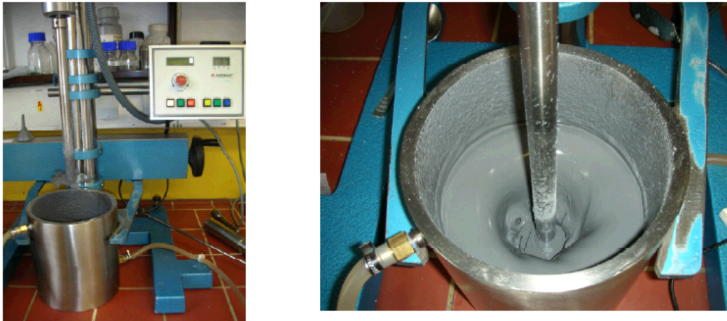
Figure 32. Procedure of the production of the final MR fluid MA 240
