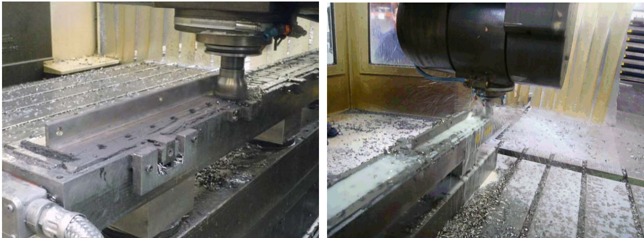
Figure 38. Photos taken during the machining of the horizontal side of the shorter profile
