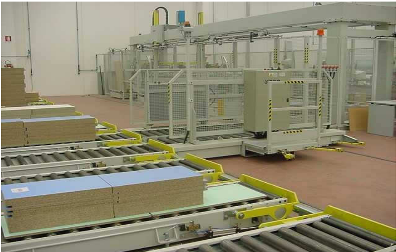
Fig. 2: An automated handling materials system for wood panels in an furniture enterprise
