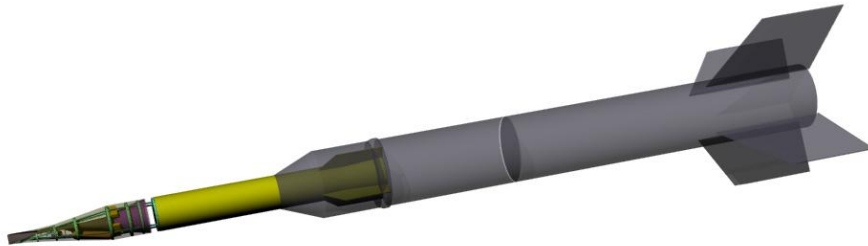
Figure 66: The ECTV concept shown mounted to the payload delivery system adopted from Shefex II. The inner and external skins and TPS have been removed from the ECTV to reveal the internal
