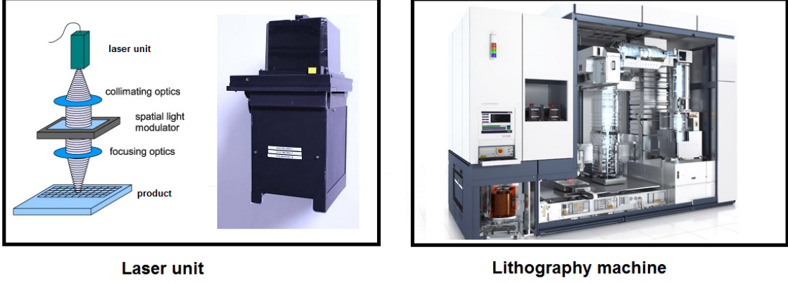
Figure 4: A laser unit in a lithography machine[1]
