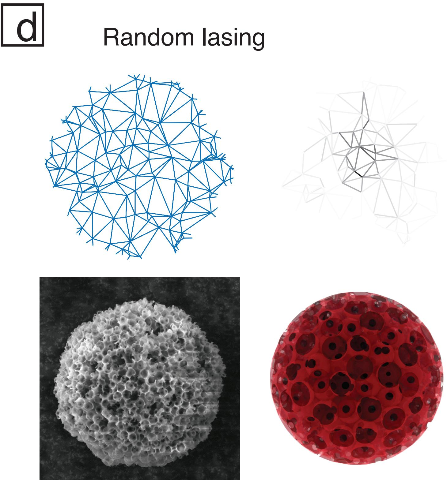
Figure 1. Panel a, a plasmonic antenna in a silicon waveguide, and two antennas to enable long-range communication between two molecules. Panel b, A single quantum dot embedded in a nanofibre and its fluorescence characterisation. Panel c, a photonic network made of linked nanofibres. Panel d, random lasing from photonic networks (top), and from 3d porous microsphere made of silk (bottom).
