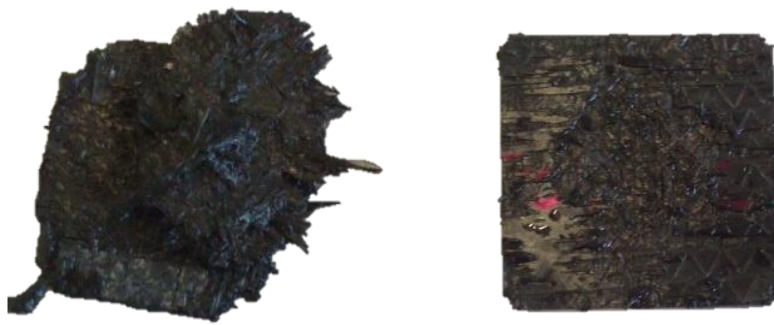
Figure 6: Size reduction of thermosets using high (left) and low (right) voltages at comparable energy input
