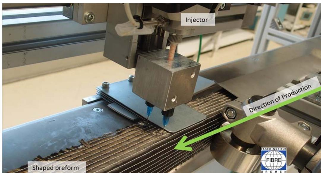
Figure 2 The chemical stitching injector assembly with the shaped and stitched preform in the foreground
