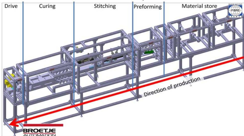
Figure 1 Automated chemical stitching and preform production line
