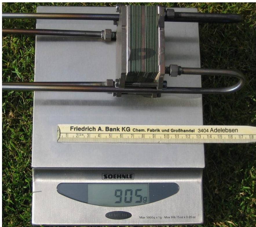
Figure 5 Planar SOFC from ALM showing stack mass of 905g
