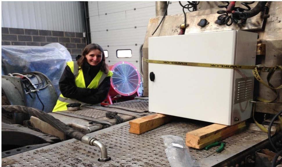
Figure 56 Fuel cell in protective box, positioned at the back of the truck cab
