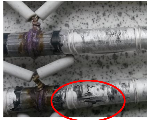
Figure 28 Polarisation measurements at reaction temperature 700°C H 2 as fuel , stack no 5. a) – single cell I-V curves, b) damaged cell no 4 showing visible crack.
