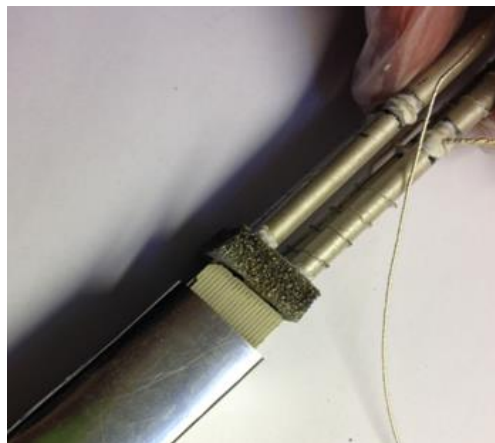
Figure 10 Stainless steel recuperator tube (30 cm long) shown as the 4-tube sub-stack assembly was inserted on the right.
