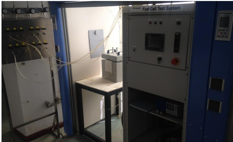
Figure 32 Test rig obtained by ADE for testing the 16 tube stack
