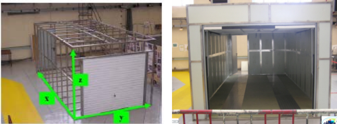
[fig.4.0] Description of GARAGE set-up as can be found at CEA Saclay (Paris). GARAGE structure showing front and service door (left) and GARAGE structure equipped with isolation sheets (right)
