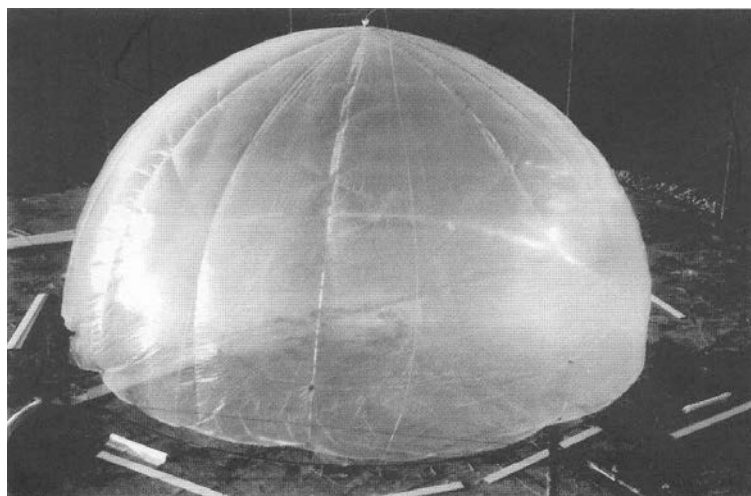
[fig.4.2] Experimental setup of open deflagration
