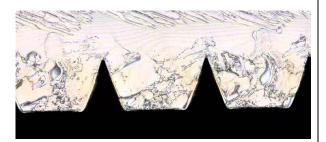
Following the successful production of samples, IFAM changed the riblet dimension specification to 51 micron height but maintained the pitch of the riblets and tip angle of 45 degrees.
