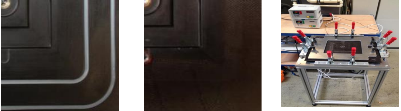
Figure 6: CFRP-tools for long-term surface tests with different surfaces: a) Gelcoat, b) C-Paper and the test rig the mold were implemented.
