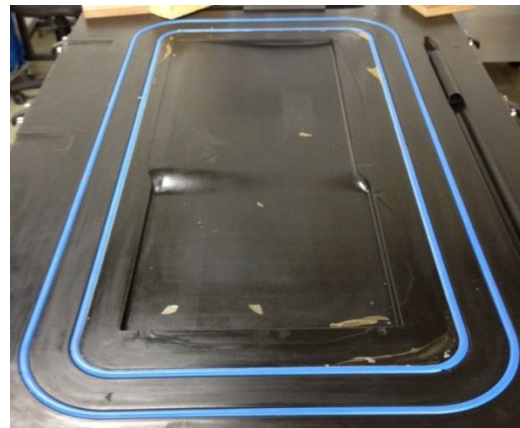
Figure 2: Sealing concept S1 with D-Section mold-sealing.
