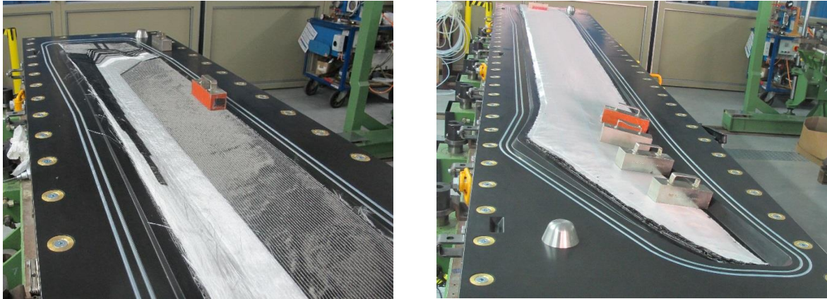
Figure 12: Layup of the full scale rotor blade.
