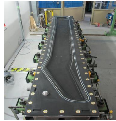
Figure 10: Manufactured set of CFRP RTM tools with integrated heating.
