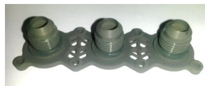
blank of connector holder – aluminum additive manufacturing
