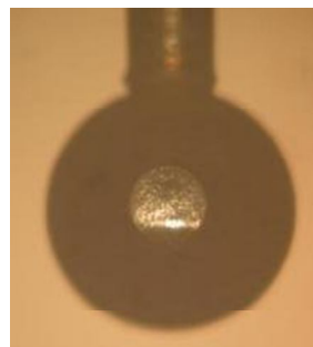
wear effect seen on ball on EHSV
