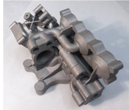
blank of housing – stainless steel additive manufacturing
