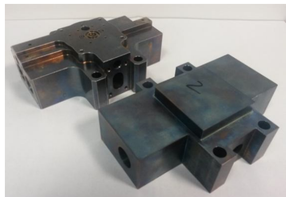
"Simplified housing" used for finishing machining tests
