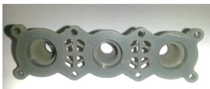
blank of connector holder – aluminum additive manufacturing
