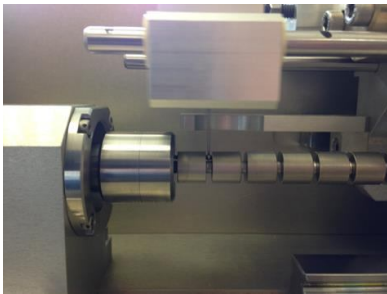
Tribologic test bench dedicated to reproduce contact ball / spool in accelerated conditions
