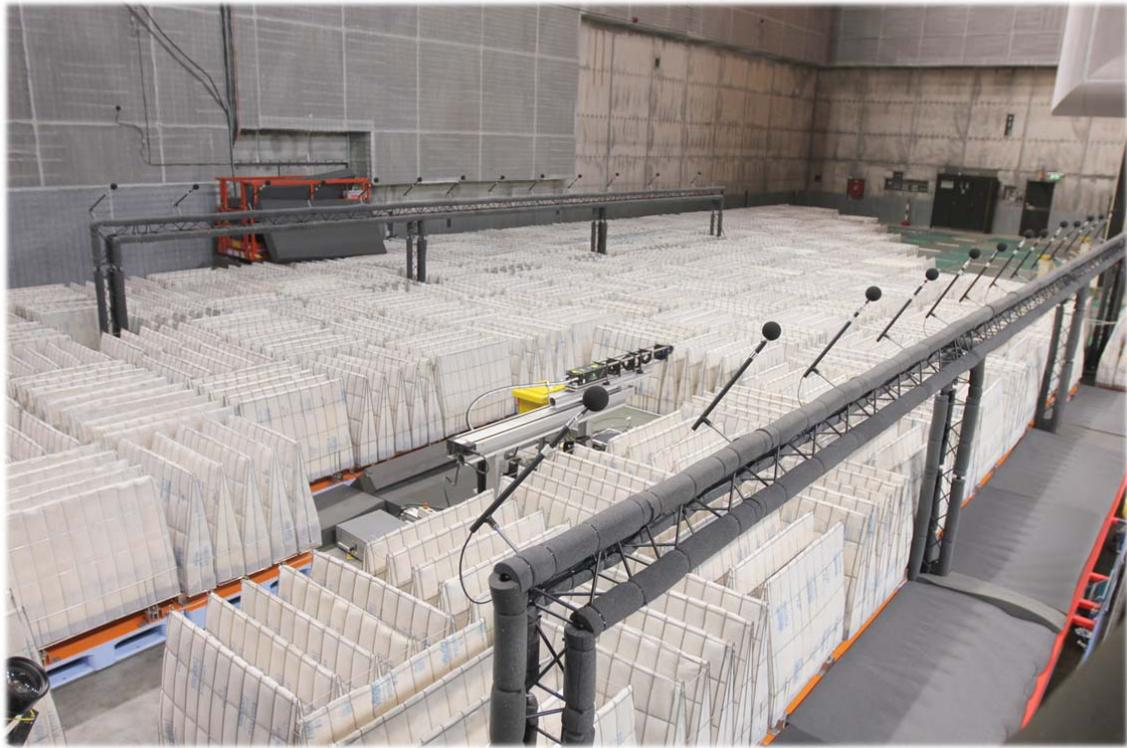
**Figure 4:** MS3 - Details of two starboard floor side line microphone lines and PIV laser unit setup
