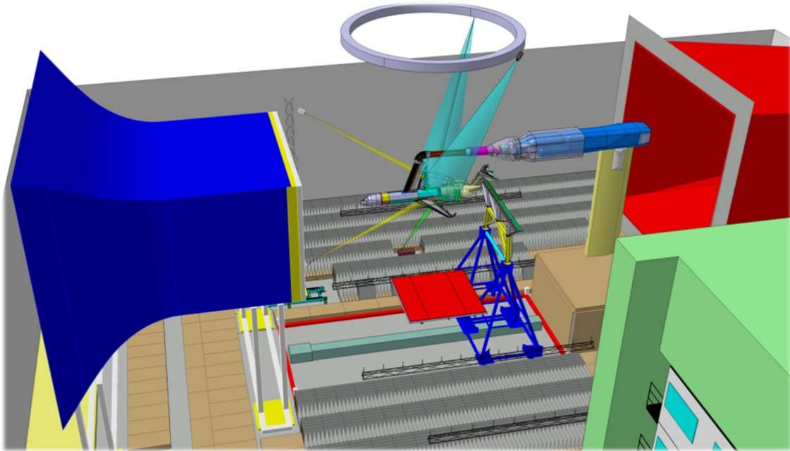
**Figure 3a:** MS3 - CAD design of test setup with inflow microphone wing, phased microphone array and out-of-flow side-line microphones on the floor
