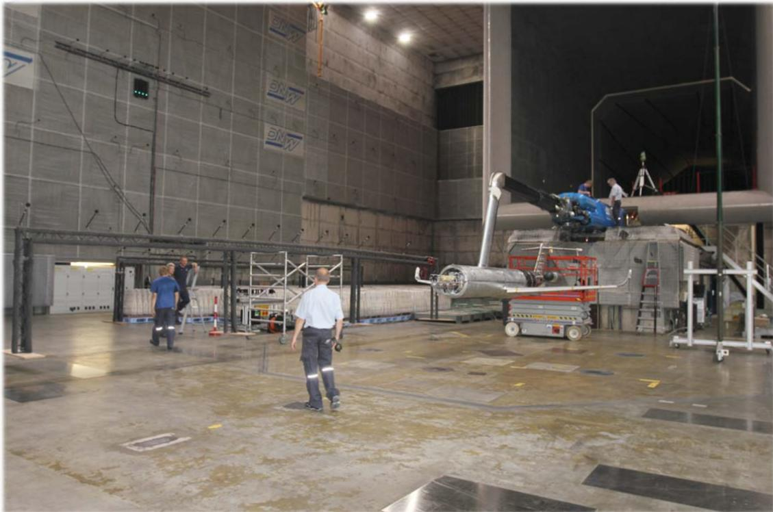
**Figure 2:** MS2 - Z08 model installation in DNW-LLF open test section
