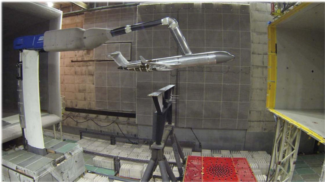
**Figure 3b:** MS3 - Z08 model in DNW-LLF open test section during aerodynamic and acoustic test
