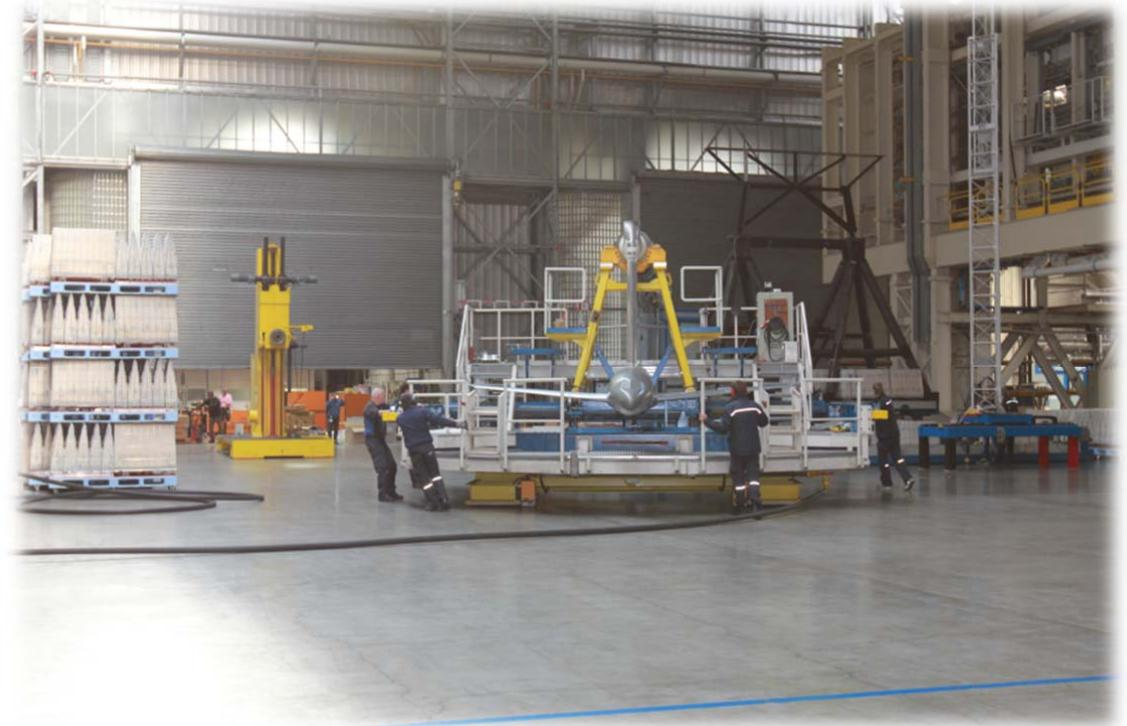
**Figure 5:** MS4 - Z08 model removal from test setup back to model hall for break down after the test
