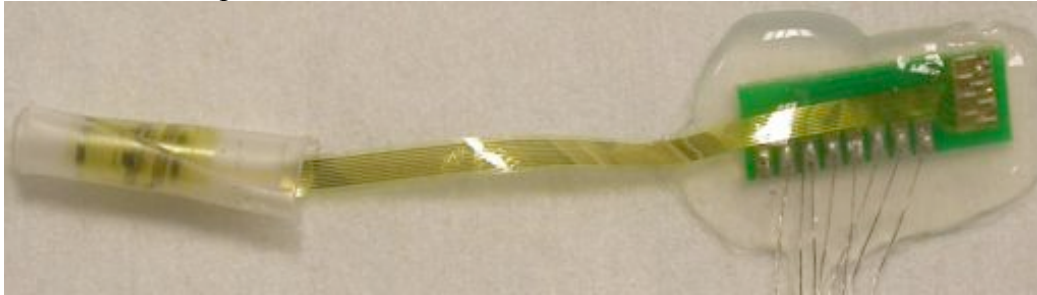
Figure 1. The neural interface with self-curling silicone cuff that is placed around the nerve bundle.
