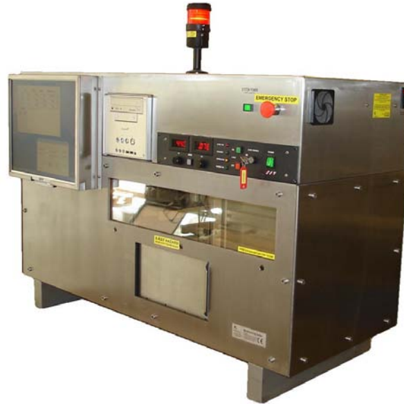
Figure 21: The SCINTAX x-rays testing facility (complete system) for evaluation and presentation of frame mode imaging detector (The system is a stand-alone system for manual insertion of a sample at a time through a sliding door in the cabinet front. There is no detector fitted).
