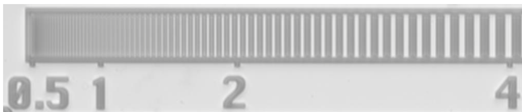
Figure 11: Vertical pattern test of the X-radia target (effective pixel size= 0.25 \mu\text{m} , 12 \mu\text{m} LSO:Tb scintillating film, M_{\text{eff}}=36 \times ).
