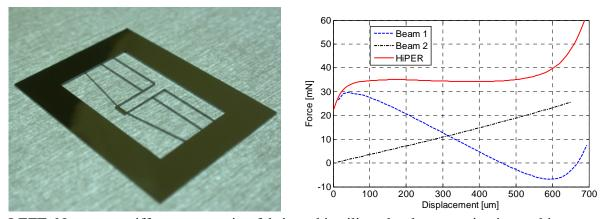
LEFT: Near-zero-stiffness suspension fabricated in silicon by deep reactive ion etching. RIGHT: FEA (finite element analysis) results showing force-displacement curves for constituent linear and non-linear elements, together with overall characteristic showing near-zero differential stiffness in central region.
