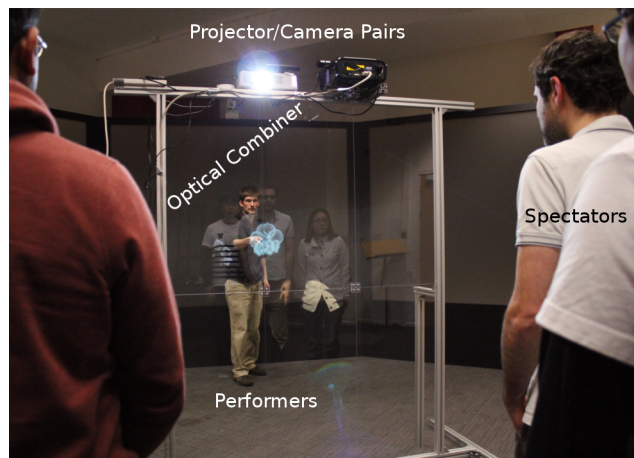
Illustration 4: Main components of the Reflets display
