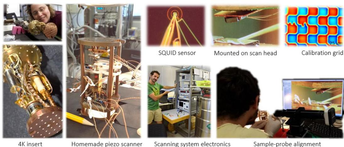
We established a functional lab oriented to sensitive magnetic imaging, and layout the foundations for scanning SQUID microscopy, including a 4K vacuum insert for variable temperature measurements in liquid helium environment. We have also designed and built the various tools required to make the microscope itself and a basic form of the SQUID probe. Preparing the microscope and scan head, which are completely homemade, is composed of many stages and has been quite a complicated task.
