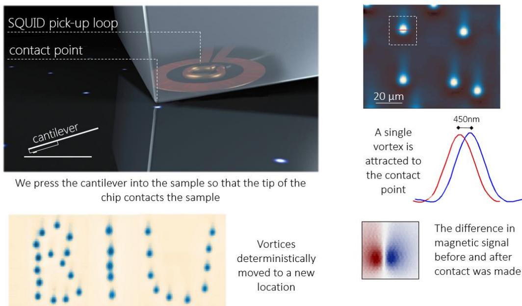
We studied the interaction between strain and nanomagnetic objects in system of vortices in a superconductor thin film. Vortices can be manipulated by applying magnetic field or current but these techniques are either non-local or confined the magnetic field strength.
