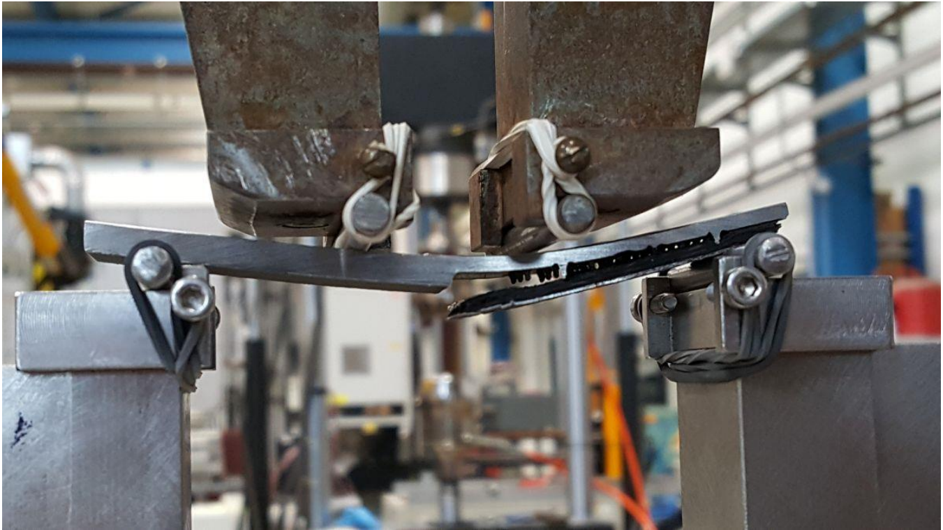
Figure 9: 4-point bending test of sub-element demonstrator
