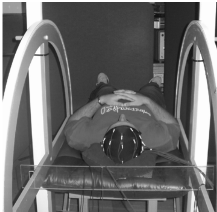
Fig. 2. The EEG signals recorded from the subject lying down between the Helmholtz coils during the ELF magnetic field exposure.
