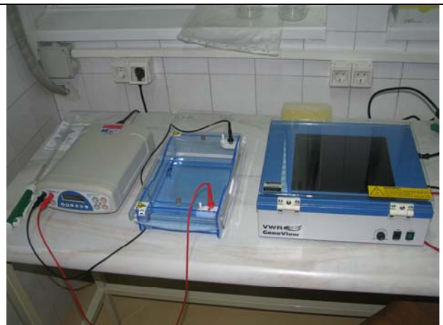
Figure 6: Power supply, Gel-electrophoresis unit and Transilluminator for visualization of the conventional PCR results.
