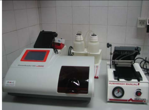
Figure 1: ELISA reader and ELISA washer for performing of ELISA technology.
