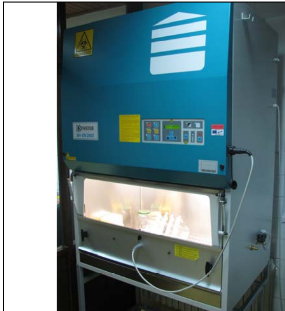
Figure 3: Laminar flows class 2 for preparation of Master Mixes in the PCR laboratory.
