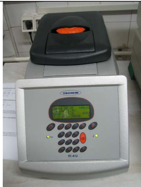
Figure 4: Conventional PCR thermocycler with 96 well microtitar format.
