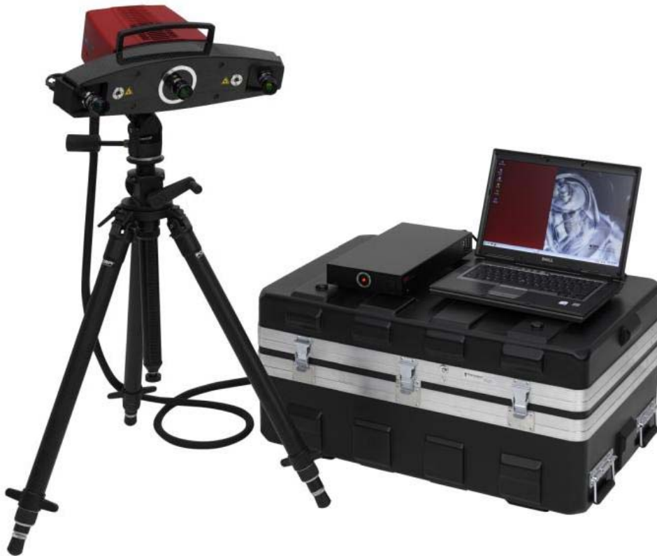
Additional stand ATOS IIe (tripod system ALFAE + 3D image processing system)
