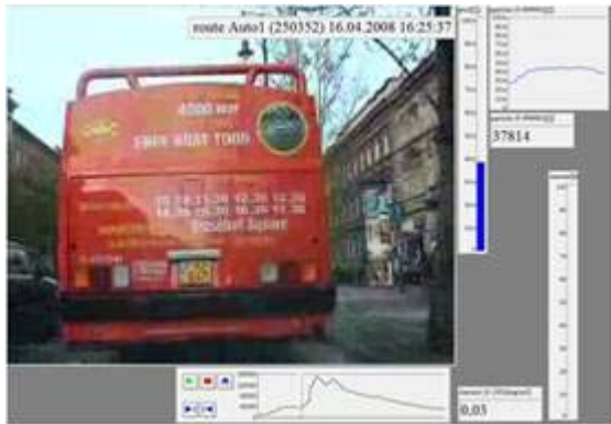
Fig. 9 – One of the measurements in a car, with real-time visualisation of particle exposure
