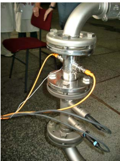
Fig.1: Online sensor device for measuring color, ph, conductivity and temperature
