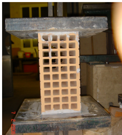
figure 2 compression test of the optimised clay brick (1 st optimisation step) in longitudinal direction
