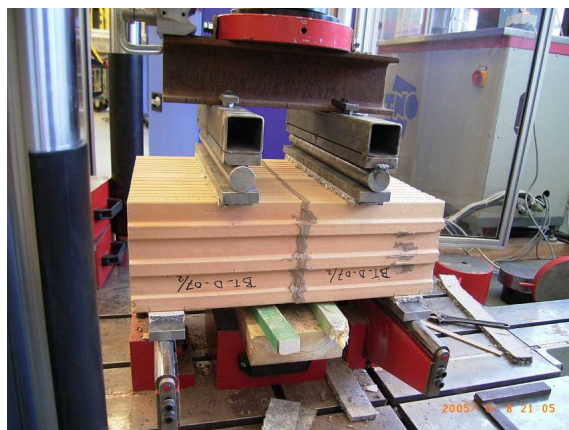
figure 1: four point bending test arrangement
