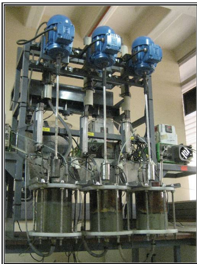
Figure 11: Bench-scale facilities used to optimize conventional tank bioleaching processes to treat Aguablanca nickel-copper concentrate and RTB-Bor copper concentrates.
