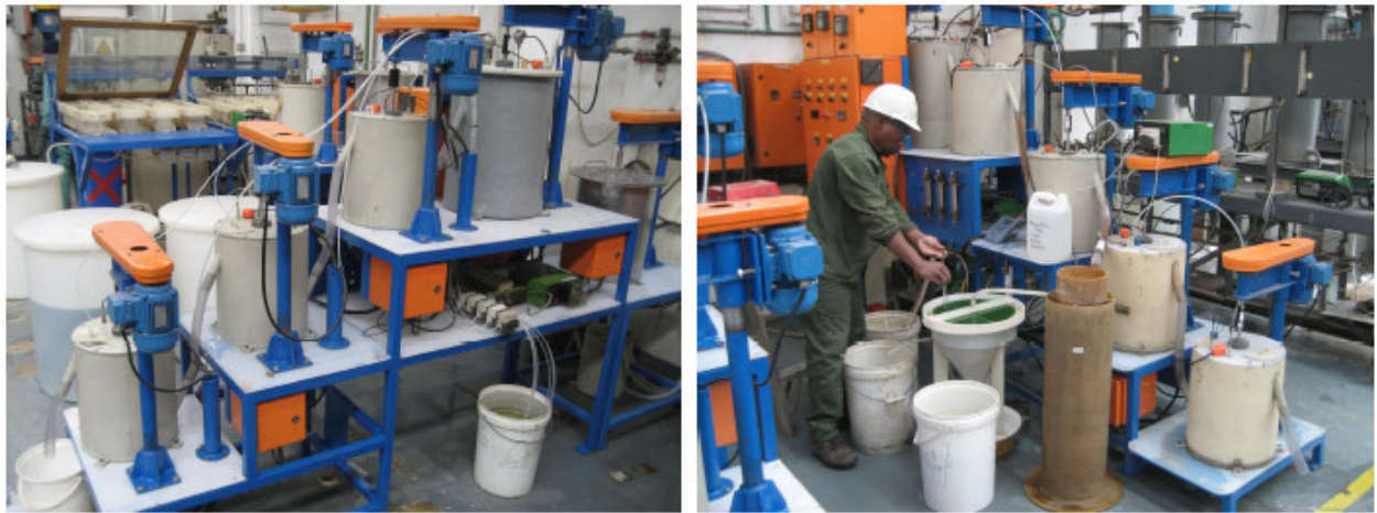
Figure 20: The integrated bioleaching pilot plant treating Aguablanca Cu/Ni concentrate.
