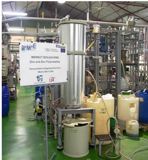
Figure 21: Flooded packed-bed bioreactor of the TR pilot plant unit using indirect bioleaching for treating a Zn/Pb concentrate.
