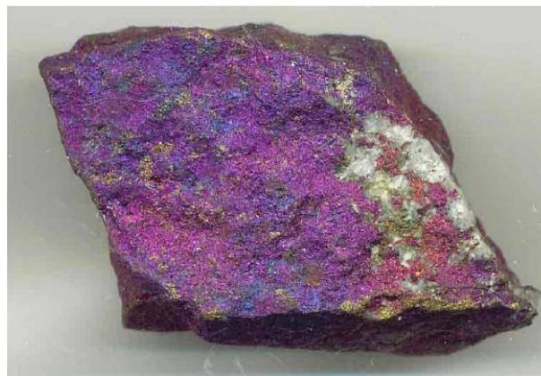
Figure 10: Chalcopyrite ( \text{CuFeS}_2 ) ore sample
