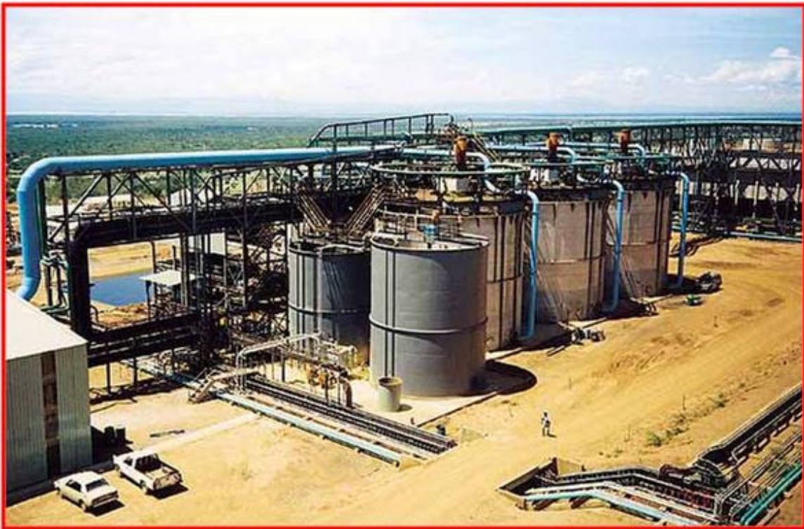
Figure 7: Bioleaching plant at the Kasese mine, Uganda, for extraction of cobalt from pyrite tailings.
