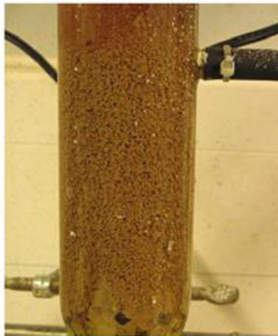
Figure 13: Indirect bioleaching process – bench-scale development of a high rate iron bio-oxidation reactor.
