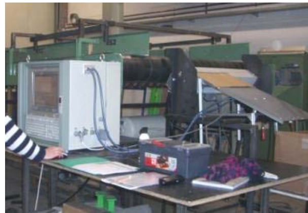
Fig.2: Unusable materials sensor (PTS/LLA)
