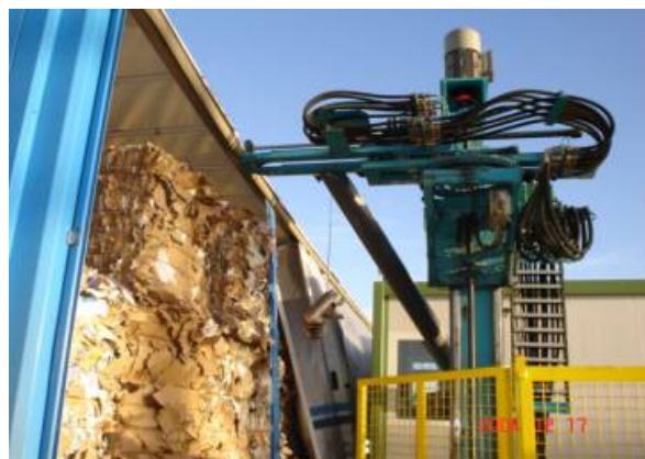
Fig.3: MONITOR sensor (CTP/Techpap)
