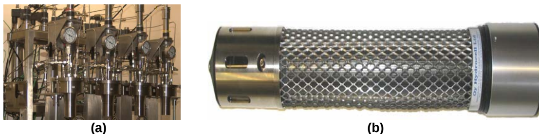
Figure 6: (a) Slurry-phase hydrogenation reactors, and (b) commercial alkaline fuel cell.
