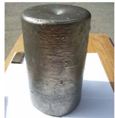
Figure 3: Recycled ingot of \gamma -TiAl produced in IMPRESS. [Courtesy: IME-RWTH]
