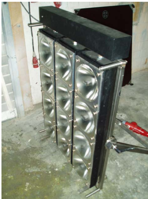
Figure: halogen lamps heat source used during the first tests with the Lock-In application (12kW)
