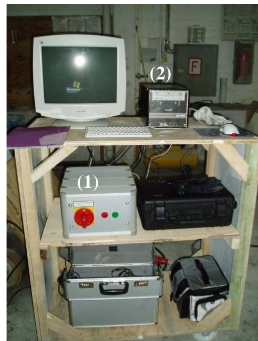
Figure: electric control (1) for the steering of the modulation of the heat source, and computer (2) with the Lock-In application.
