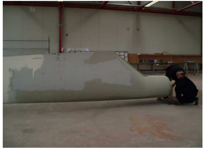
Picture: Inspection of a complete rotor blade using a construction blower blowing hot air into the rotor blade.
