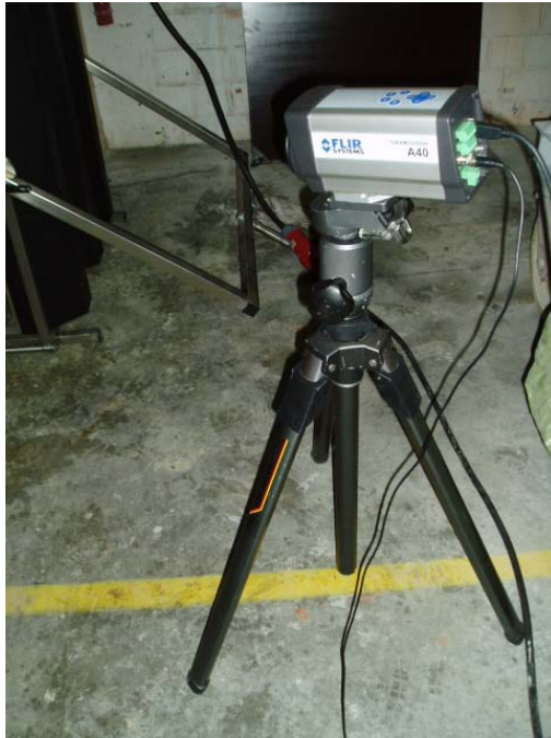
Figure: digital picture of the thermographic camera used for taking the Lock-In images above (FLIR Camera A-40).
