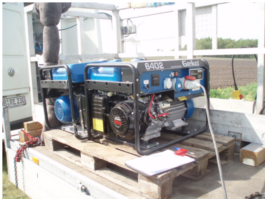
Fig.: two diesel generators provided the required power for the platform and the heat source
