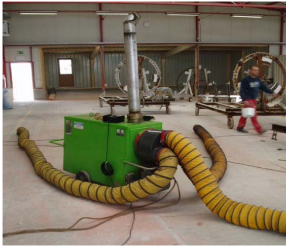
Picture: Inspection of a complete rotor blade using a construction blower blowing hot air into the rotor blade.
