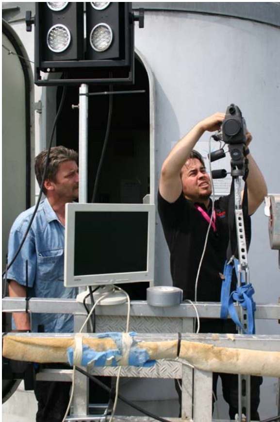
Fig.: the IR-camera and other components had to be fixed to the platform using the custom made supports
