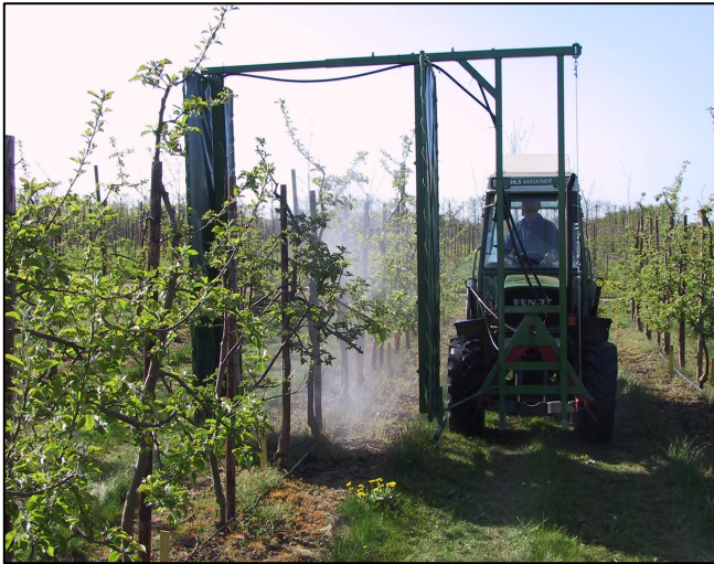
Figure 15. Tunnel sprayer with 8 nozzles, Tee-jet 110-02. Water volume: 1000 l ha -1 . Sprayer made special for this trial as alternative to knapsack spraying.
