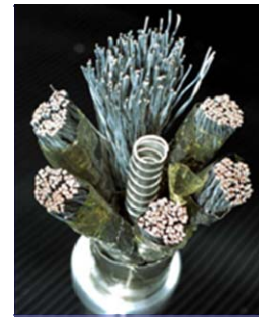
Real superconducting cable modelled by a homogenization technique (KMM-NoE)
