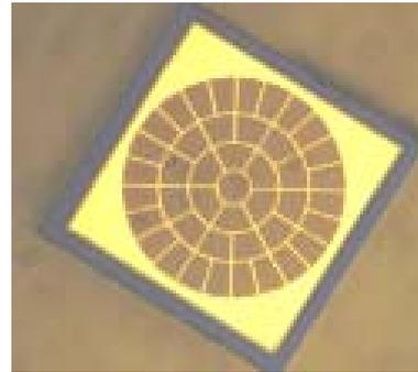
Fig. 3 Left, result of a quantum mechanical calculation in search of an intermediate band material. Right, Quantum dot intermediate band solar cell test sample.
