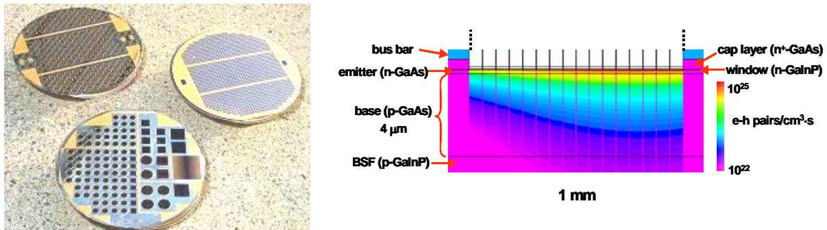
Fig. 1 Left: dual junction solar cells in their wafer. Right: computer simulation of the photogenerated current in a concentrator solar cell under non uniform illumination.
