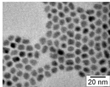
Fig. 4: Left, flat concentrator. At the bottom edge of the concentrator silicon cells are located. Right, PbSe quantum dots synthesized to form aggregates with CdSe QDs as basis for an up-converter material.
