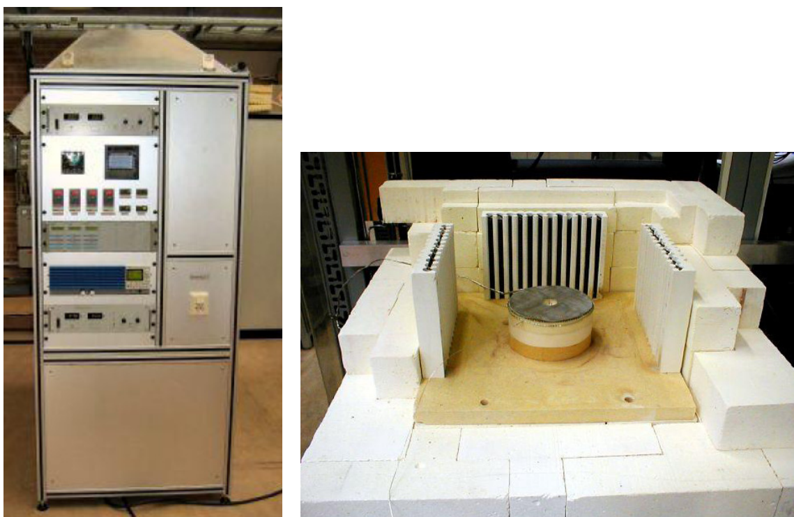
Figure 3: Front panel of the test-rig developed by ECN for planar cells (left); heating elements and housing for planar cells (right)
