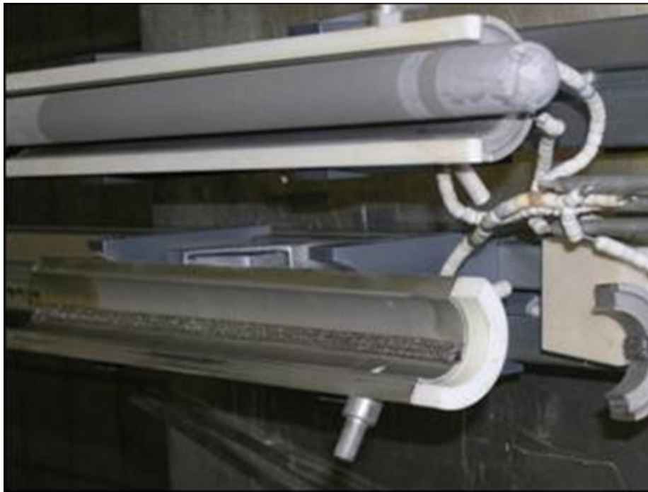
Figure 10: Siemens SOFC test-rig for long-term tests
