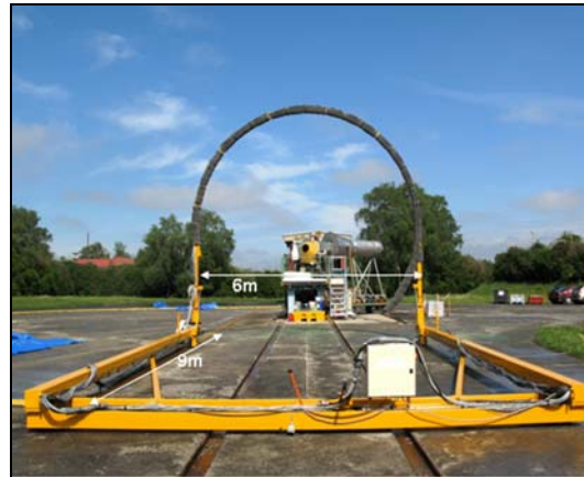
Figure 12 ONERA acoustic antenna for static tests
