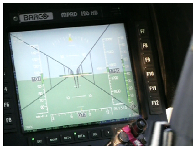
Figure 5 View of the tunnel-in-the-sky guidance system installed in the EC135
