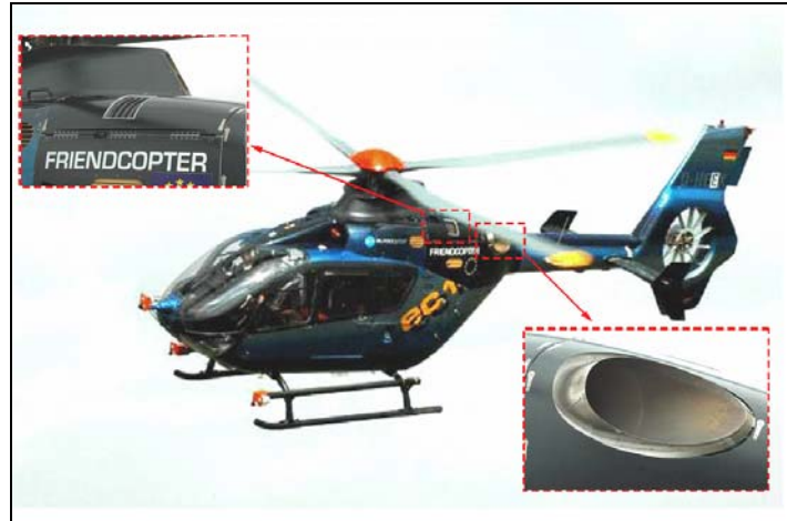
Figure 10 Two technologies tested on the EC135 with Arrius2 engines: static silent air intake and quiet ejector
