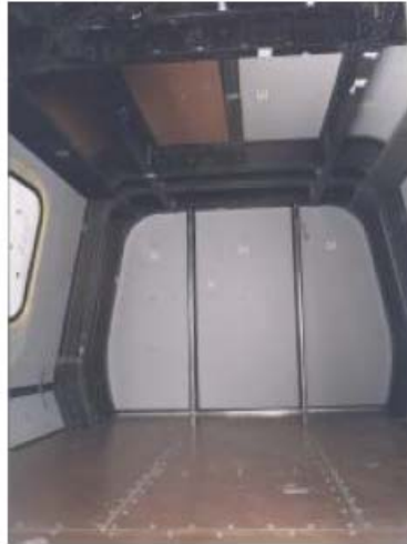
Figure 25 Tests of active cabin panels in ONERA cabin mock-up VASCO
