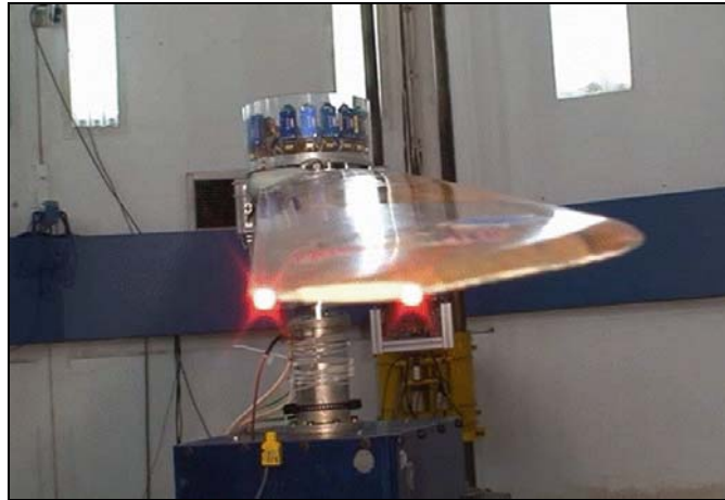
Figure 26 Active twist blade tested in DLR's spin facility
