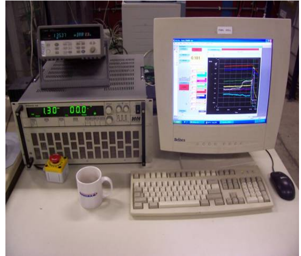
Figure 11b. Fuel cell control and electronic load
