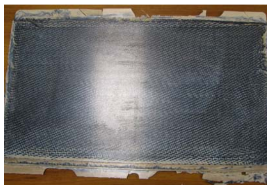
Fig. 17 : PPS/C injected laminate _EADS IW
