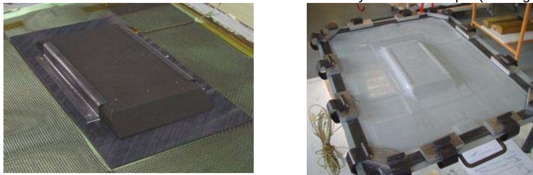
Fig. 26: Dassault Av._ Carbon foam blocks used as tool to hold stiffeners in place (left). Silicone membrane used to ensure good pressure distribution (right).
