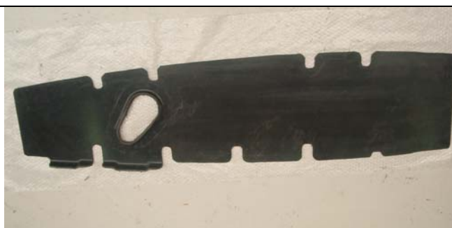
Fig 33: consolidated PEEK/AS4 rib & feet- Eire Composites
