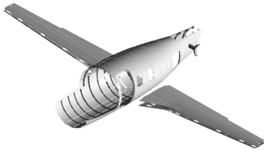
FIG 3. parts assembled by FSW technology on Eclipse 500 aircraft
