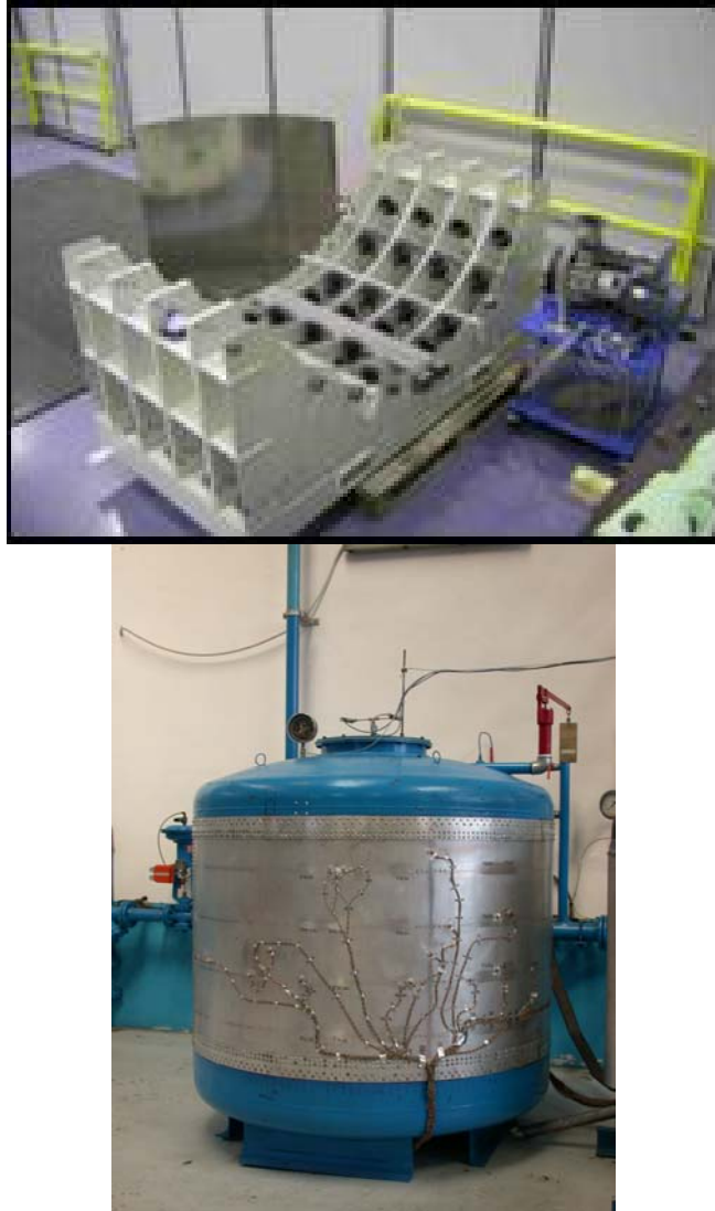
FIG 40. clamping tool design (Dassault Aviation) – left P180 fuselage barrel test – right
