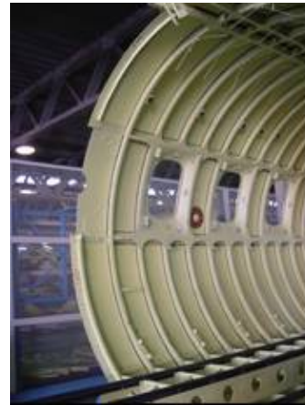
FIG 4. stringerless fuselage architecture on P180 business aircraft
