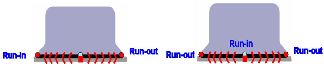
FIG 15. welding sequences tested for the clip welding
