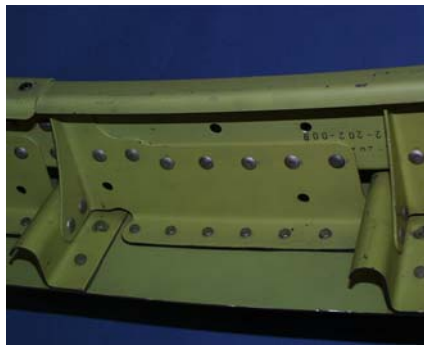
FIG 2. clip-frame-stringer to skin joining
