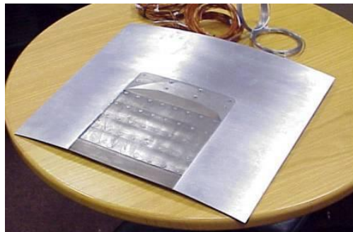
Figure 9 Post ADVACT wind tunnel model of interlocking slats variable area nozzle
