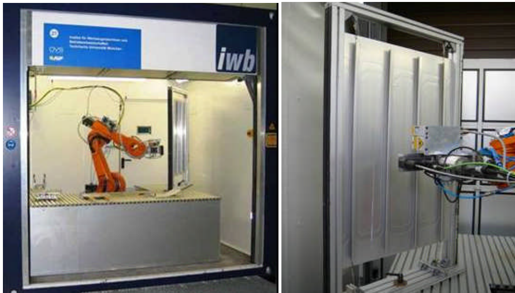
Figure 1.2.2.5: Completed prototype of LBF forming unit
