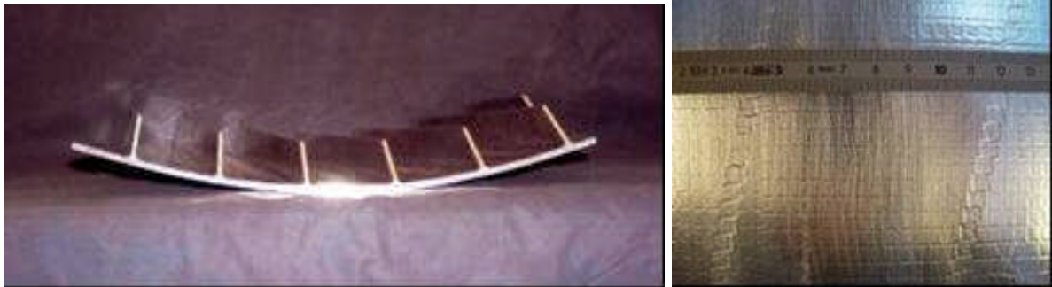
Figure 1.2.2.3: Thick walled stiffened panel after successful LPF processing
