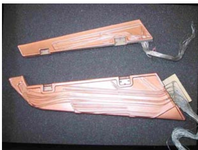
Pressure Plotting: Innovative technology: main body and elevator covered with copper
